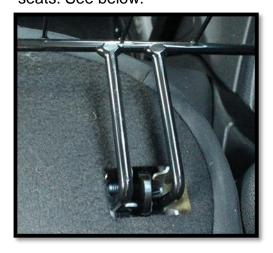
On top of the guard are two metal wrap around clips, one on either side. These will fit onto the bolts from the fittings on the handles
