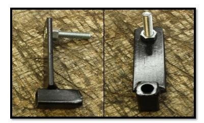
The fittings supplied will fit in place of the handles above the rear passenger doors. Remove the screws from the front side of the handles and screw in the two fittings, one on each side. They will look like this in place:
